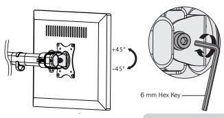
It may be necessary to slightly loosen or tighten the adjustment screw, depending on the weight of display installed.
