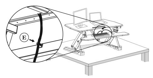
Stick the WIRE CLIP (E) to back of the crossbar. Use this clip to route cables from keyboards, mice and monitors through the <u>REAR</u> of the desk.
