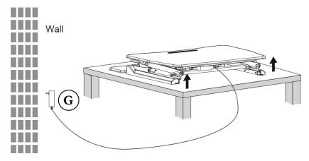
**STEP 4.** Press the UP button on the controller to lift the AIRLIFT™ DESK (A).
