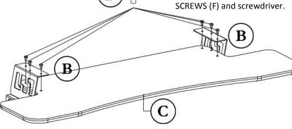
**STEP 6.** Hook BRACKETS (B) over the bolts on the inner legs of the AIRLIFT™ DESK (A). Tighten bolts clockwise with included ALLEN WRENCH (D).
