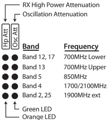
The "LEDS" on the face of the booster indicate operating gain state.
