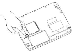
Sample unlocking the battery
