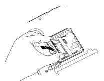
Sample inserting the memory module
