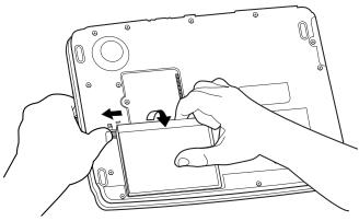
Sample removing the battery
