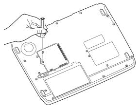
Sample removing the expansion module memory slot cover
