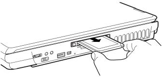
Sample removing a PC Card
