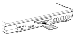
Sample inserting an xD-Picture Card
