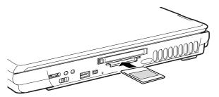
Sample inserting an SD Card
