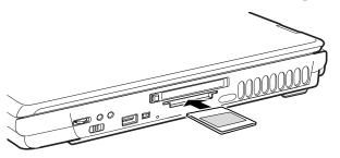
Sample inserting an Smart Media Card
