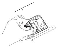
Sample removing the memory module
