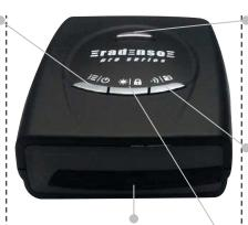
Alphanumeric Display Radenso Pro-M will show selected display mode, visual alerts and Display/Alert Lockout Button text messages.
