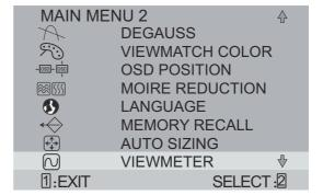
2 To select a control you want to adjust, press the arrow buttons on the front control panel of your monitor and scroll through the choices. When the control you want is highlighted, press button [2].
