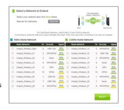
If you fail to find any wireless networks, or your signal strength is below 70%, try moving the Range Extender closer to the wireless network that you are trying to repeat and click SCAN again.
