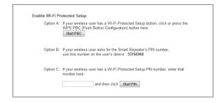
Option A: Push button: You may push the WPS button on the web menu or use the physical button on the back of the Range Extender.
