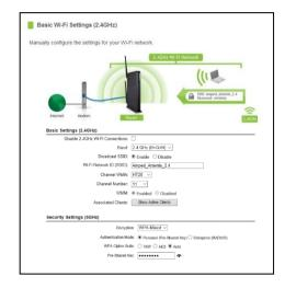
Wireless Network ID (SSID): The name of your 2.4GHz wireless network.
