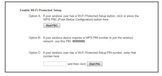
**Option A:** Push button: You may push the WPS button on the web menu or use the physical button on the back of the Access Point.
