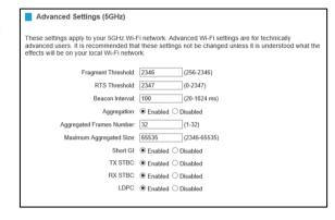
**Beacon Interval:** Indicates the frequency interval of the beacon. A beacon is a packet broadcast by the Access Point to synch the wireless network.
