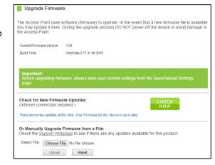
Manual Firmware Upgrade: In the case that the Range Extender does not have access to the Internet, you can manually upgrade the firmware by downloading the firmware file from the Amped Wireless Elite Support website. The firmware update is downloaded as a zip file and you will need to have an unzipping program to open the file. Inside the file will be a text document with details on the current firmware release and instructions on how to upgrade the firmware.
