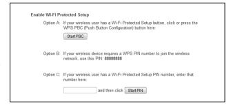
**Option A:** Push button: You may push the WPS button on the web menu or use the physical button on the back of the Router.
