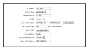
**Set Static DHCP:** This allows specific devices to be given a specific IP address each time the device connects to the network. The DHCP server will always assign the same IP address to the same device. This feature is often used for shared devices such as network printers or servers.
