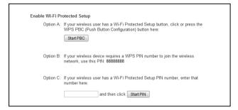
**Option A:** Push button: You may push the WPS button on the web menu or use the physical button on the back of the Router.
