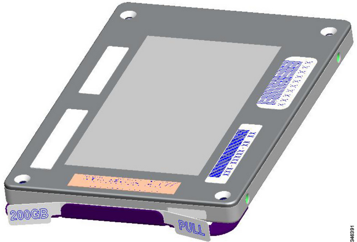
Figure 6-8 Solid State Drive
