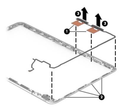
Reverse this procedure to install the WLAN antenna cable.
