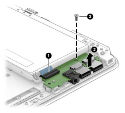
Reverse this procedure to install the I/O board.
