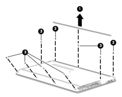
3. Slide a nylon flake tool around the edge of the base enclosure to loosen it, taking care not to damage the internal clips, and then remove the base enclosure.
