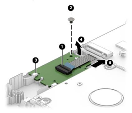
Reverse this procedure to install the SD card reader board.
