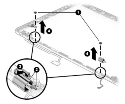
5. Remove 4 Phillips 2.0x2.5 screws from the display panel (1), and then lift the display panel (2) to remove it.
