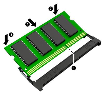
3. Gently press the memory module down (3), applying pressure to both the left and right edges of the memory module, until the retention clips snap into place.
