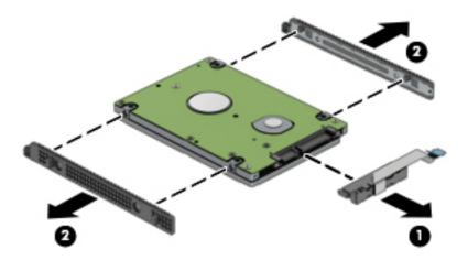
Reverse this procedure to reassemble the hard drive.
