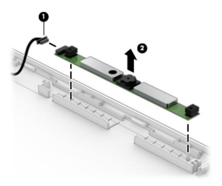
Reverse this procedure to install the webcam.
