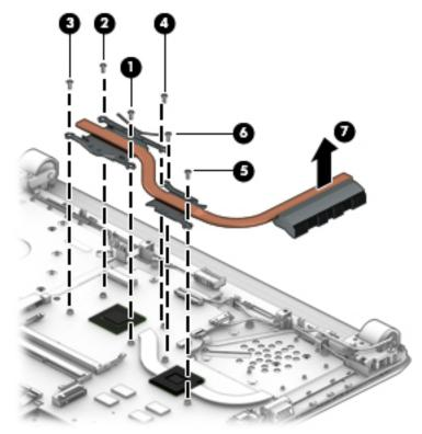
• **Discrete graphics** Thermal paste is used on the processor and associated heat sink area (1)(2), as well as the graphics chip and associated heat sink area (3)(4).
