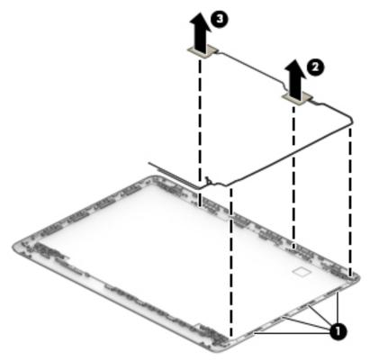
**6.** To remove the display/camera cable, remove the cable from the clips built into the side of the display enclosure **(1)**, and then remove the cable from the display enclosure **(2)**.
