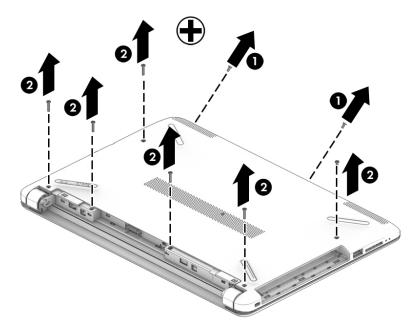
**3.** Use a plastic, non-marking tool **(1)** to pry the bottom cover from the computer **(2)**.
