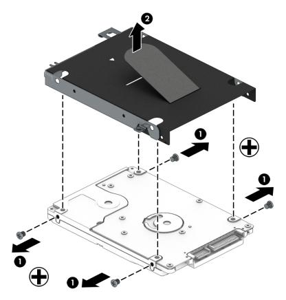
Reverse this procedure to reassemble and install the hard drive.
