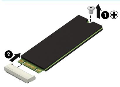
Reverse this procedure to reassemble and install the solid-state drive.
