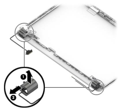
c. Remove the two Phillips PM2.0×3.0 screws (1), and then lift the top display hinge (2) off the display.
