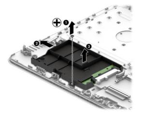
Reverse this procedure to reassemble and install the solid-state drive/eMMC adapter bracket.
