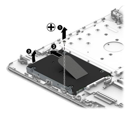
**3.** To remove the hard drive bracket from the hard drive, remove the four Phillips PM3.0×3.0 screws **(1)** that secure the bracket to the hard drive.
