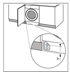
**15.** Screw the spacers in as per the dimensions.
