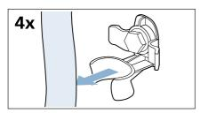
2. Use a WAF13 spanner to undo and remove all four transport lock bolts.
