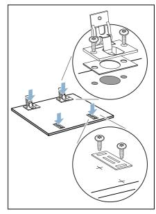
**10.** Put the hinges in the appliance (1 + 2), push on the cover panels (3) and screw them in place (4).
