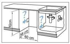
Lay the mains cable and the hoses. Push the appliance in, moving the mains cable and the hoses with it.
