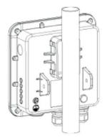
2 Insert the straps in the slots on the device and wrap around the pole
