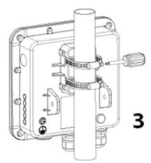
Fasten the screws and make sure the device is firmly attached to the pole
