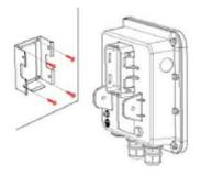
2 Attach device to the mounting bracket
