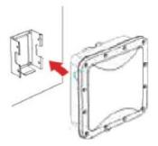
Insert screws in the slots on the mounting bracket
