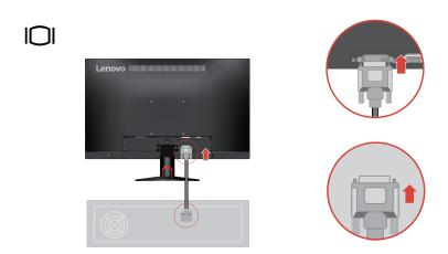
4. Connect the digital to the DP connector of the monitor and the other end on the back of the computer.
