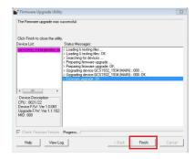
After a successful completion, the GCS1932/1934 will exit the Firmware Upgrade Mode and resets itself.
