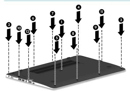
NOTE: There are five different sizes of rubber screw covers. Be sure that you reinstall them over the correct screws, as shown in the following images.
