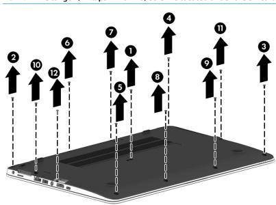
**NOTE:** The longer (Phillips M2.0x7.0) screw is located under the SD card reader.
