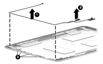
If it is necessary to replace the WLAN antenna cables, peel the transceivers from the top of the display enclosure (1), remove the antenna cables from the routing path on the sides of the display enclosure (2), and then remove the antenna cables (3).
