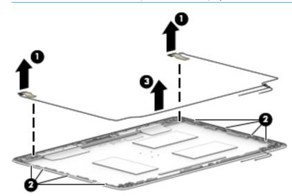
**NOTE:** The WLAN antennas are spared with the display enclosure.
