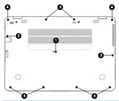
NOTE: If installing new rubber screw covers, carefully inspect for adhesive tape liner inside the cap and remove if present.
