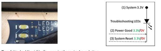
These lights should be visible after removing the service door or bottom cover. Consult with support for platform-specific locations of the lights.
