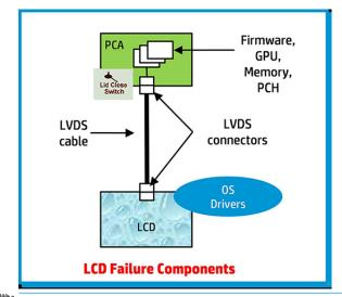
NOTE: The lid close switch is a Hall-effect sensor located in the top cover. When the display is closed, the sensor acts like a switch. A notebook can force a video output to an external monitor, or go to hibernation or standby mode through power management. If the display screen does not light up when the display is open, the lid close switch (Hall-effect sensor) could be faulty.
