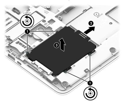
**4.** To remove the hard drive cover from the hard drive, remove the 4 Phillips M3.0×3.0 screws **(1)** that secure the cover to the drive, and then lift the cover up and off the hard drive **(2)**.
