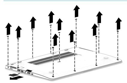
3. Remove the 11 Phillips M2.5x5.0 screws (1) - (11) and the Phillips M2.0x7.0 screw (12) in the order shown in the following image.
