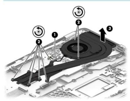
2. Discrete graphics models: The thermal material must be thoroughly cleaned from the surfaces of the heat sink and the system board components each time the heat sink is removed. Replacement thermal material is included with the heat sink, processor, and system board spare part kits.
