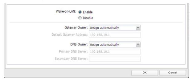
Wake-on-LAN is now enabled. As long as the TeraStation is connected to a power source and the network, you can turn it on remotely.
