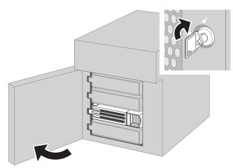
**2** The failed drive's status LED will be glowing red. Push its unlock button and swing the lock mechanism out.
