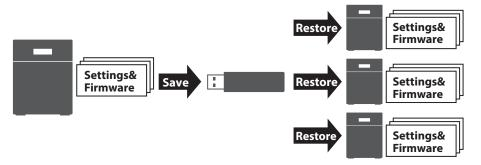
Make a note of the drive configuration (number of drives, RAID, LVM, etc.) of the TeraStation whose the settings were saved. Make sure that any TeraStation that you apply these settings to has exactly the same drive configuration before you apply the settings. If the drive configuration is different, you may get unexpected results.
