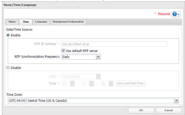
By default, the TeraStation adjusts its clock automatically by using a default NTP server. This NTP server belongs to Internet Multi Feed Inc. For more information, visit http://www.jst.mfeed.ad.jp.
