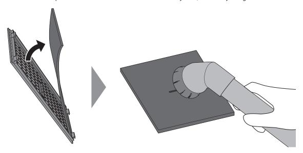
$\boldsymbol{4}$  When cleaning is finished, return the filter and the front cover.
