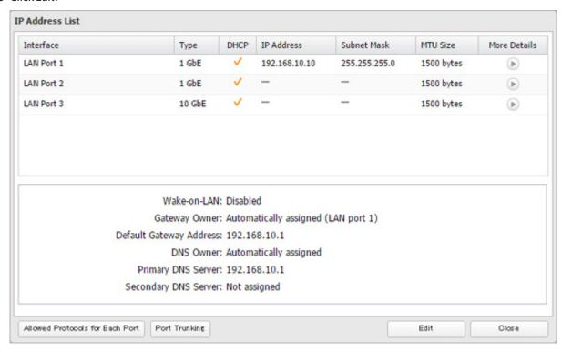
Clear the "DHCP" checkbox and enter the desired IP address and its subnet mask.
