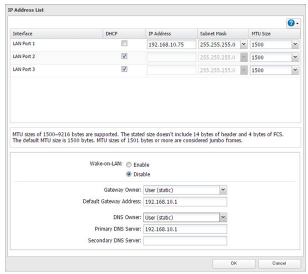
5 Select "User (static)" for both "Gateway Owner" and "DNS Owner" options from the drop-down list, then enter the desired default gateway address and DNS server addresses.
