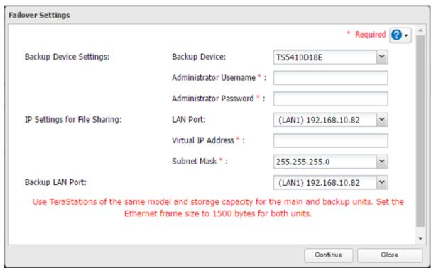
**5** Select the LAN port to be used for sharing files and enter a virtual IP address and subnet mask.
