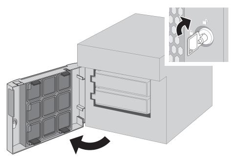
$\boldsymbol{2}$  Remove the front cover while holding the hook downward.
