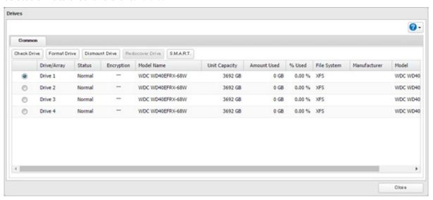
**4** The S.M.A.R.T. information for the drive will be displayed. Different information may be displayed depending on the brand of drives in your TeraStation. Critical attributes are displayed in bold. Attributes with current value less than or equal to the threshold value may be significant. If an attribute reports a failure, or has had one in the past, it will be displayed in the status column.
