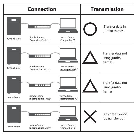
**Note:** Make sure the TeraStation's MTU size is smaller than the hub or router's. Larger MTU sizes may not transfer the data to the TeraStation correctly.
