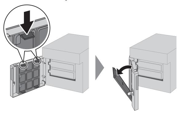
Remove the dustproof filter from the front cover and clear any dust, such as by using a vacuum cleaner.
