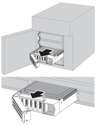
Insert the new drive into the empty slot. Slide the drive in with the locking mechanism open.
