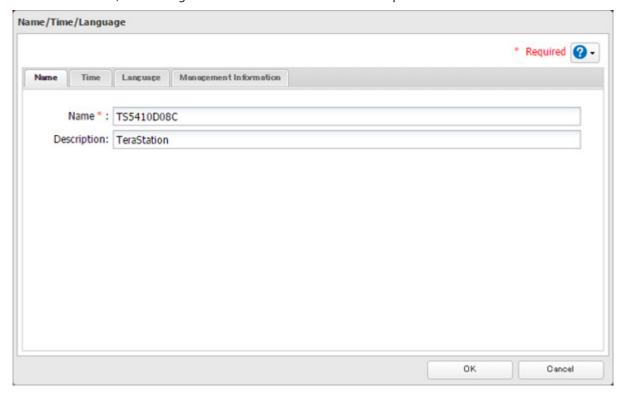
**5** Click the *Time* tab. Enable the NTP server and select the "Use Default NTP Server" checkbox.
