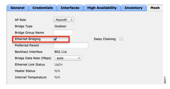
Daisy chaining should only be enabled on a Slave AP that is configured as a Bridge Mode Root Access Point, for all other daisy-chaining configurations, daisy chaining does not need to be enabled. To enable Daisy Chaining from the WLC GUI, navigate to the **Wireless > Access Point >**AP NAME > Mesh tab, and then check the Daisy Chaining check box.
