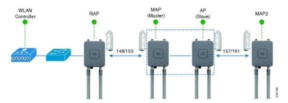
High gain directional antenna should be used in typical serial backhaul deployments. In addition, "Preferred Parent" configurations should be used to create serial backhaul mesh networks.
