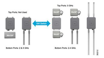
Please note that Antenna Band Mode is only available on the 1532E model, with external antennas; the 1532I has an internal antenna and does not require additional antennas.
