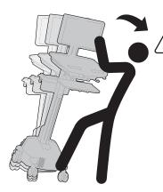
Warning: When the height adjustment and assembly are at maximum height this creates a tipping hazard. Lower work surface before moving cart. Failure to follow these instructions may result in equipment damage or personal injury.
