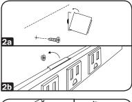
3 Clip Mounting (Style B): Pre-drill holes in the mounting surface, if necessary. Thread #8-32 screws onto the hex nuts. Drive screws through the centers of the mounting clips and into the mounting surface 3. Place the Power Strip inside one edge of the mounting clips, then snap the Power Strip into place 3.
