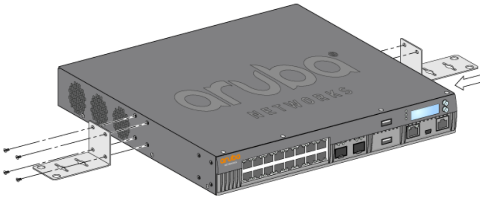
Figure 10 Attaching the Wall Mount Brackets
