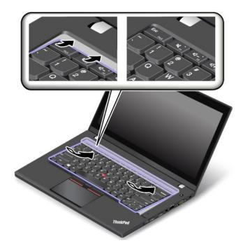
3. Ensure that the screw heads are exposed completely. Otherwise, reveal the screw heads by sliding the keyboard frame forward with the flat end of the keyboard multi-tool.
