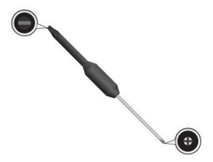
5. To reveal the screw heads beneath the keyboard frame, use the flat end of the multi-tool in the shipping package of the new keyboard to slide the keyboard forward by 2.5 mm (0.1 inch).
