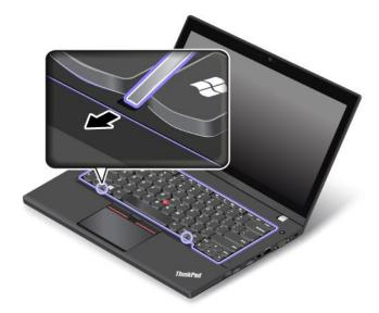
6. Insert the flat end of the keyboard multi-tool into the sides of the keyboard as shown to push the keyboard frame backward. Ensure that there is no gap between the keyboard frame and keyboard bezel.
