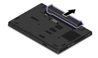
6. Insert a new battery until it clicks into place. Ensure that the battery latches are in the locked positions.
