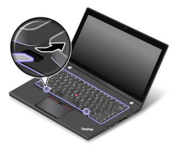
4. Tighten the screws with the cross end of the keyboard multi-tool to secure the keyboard in place.
