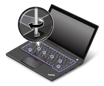
5. Slide the keyboard frame backward by 2.5 mm (0.1 inch) with the flat end of the keyboard multi-tool to hide the latches of the keyboard frame under the keyboard bezel.
