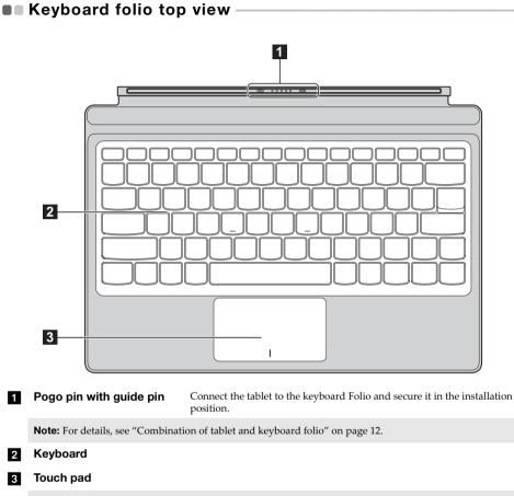
**Note:** When the Keyboard folio is rotated to 360 degrees after connection with a computer, the Keyboard and touch pad will be locked automatically.
