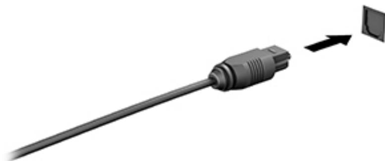
2. Connect the other end of the cable to the digital speakers.
