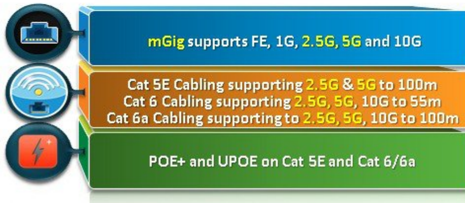
Figure 53: Cisco Multigigabit distance limitations
