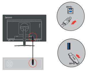
8. Connect one end of the USB cable to the USB downstream terminal on the side of the monitor, and connect the other end of the USB cable to an appropriate USB port on your device.
