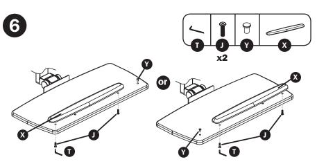
The keyboard Wrist Rest attaches to the left or right side of the Keyboard Shelf to allow for a mouse. If the Wrist Rest is not needed, insert the Plugs to fill the holes.
