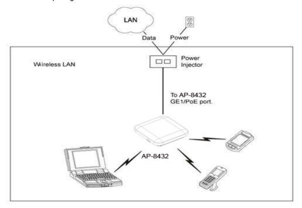
The Power Injector can be installed free standing, on an even horizontal surface or wall mounted using the Power Injector's wall mounting key holes. The following guidelines should be carefully followed before cabling the Power Injector to an Ethernet source and an Access Point:
