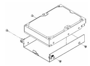
8 Insert the loaded hard drive tray into the empty hard drive bay and tighten the screws using the 3mm Hex Tool.
