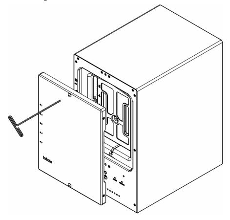
Remove the Waterproof Drive Cover using the 3mm Hex Tool.
