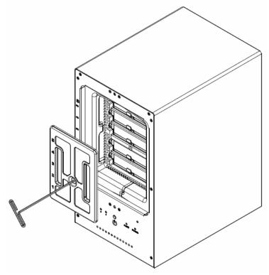
10 Install the Front Cover to finish the installation and protect the drives from fire. Keep the Hex Tool nearby for future use. A magnet is provided to attach the Hex Tool to the back of the ioSafe or some other convenient location.
