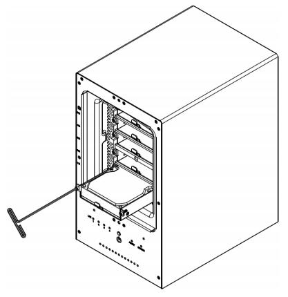
Important: Make sure the tray is pushed in all the way. Otherwise, the hard disk might not be able to function properly.
