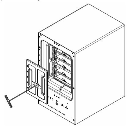
Remove the Drive trays using the provided 3mm Hex Tool.
