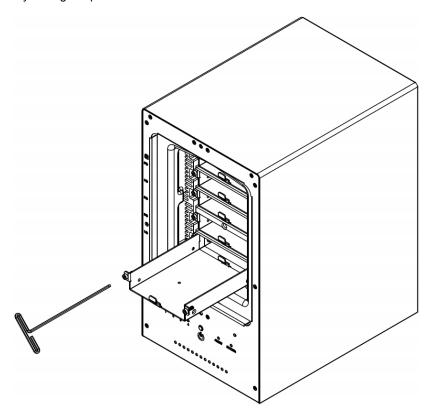
7 Install a compatible Hard Drive into each Drive Tray using (4x) Drive Screws and a Phillips screwdriver. (Please visit www.iosafe.com for compatible hard drives models.)
