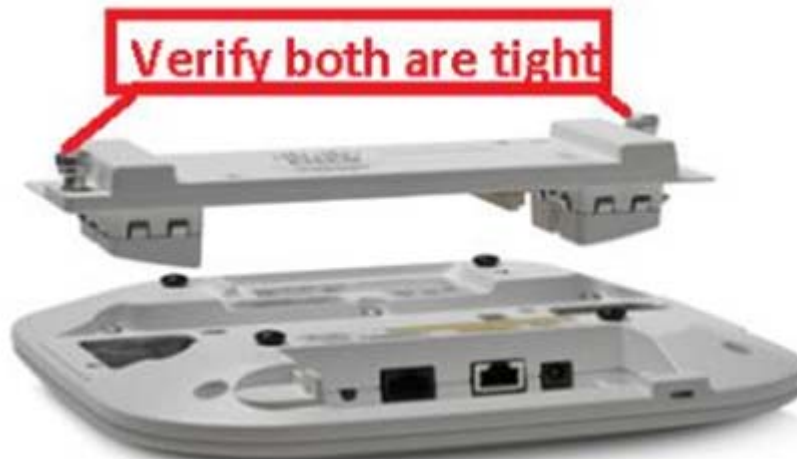
Figure 77 Both Thumbscrews Need to be Tight or Power is Not Applied
