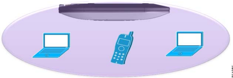
Figure 73 Coverage is Optimized for Ceiling Placement and Radiates Omni-Directionally
