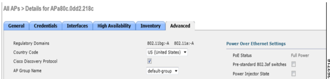
Figure 100 AUX port is active when PoE status is at FULL power or when a local power supply is used
