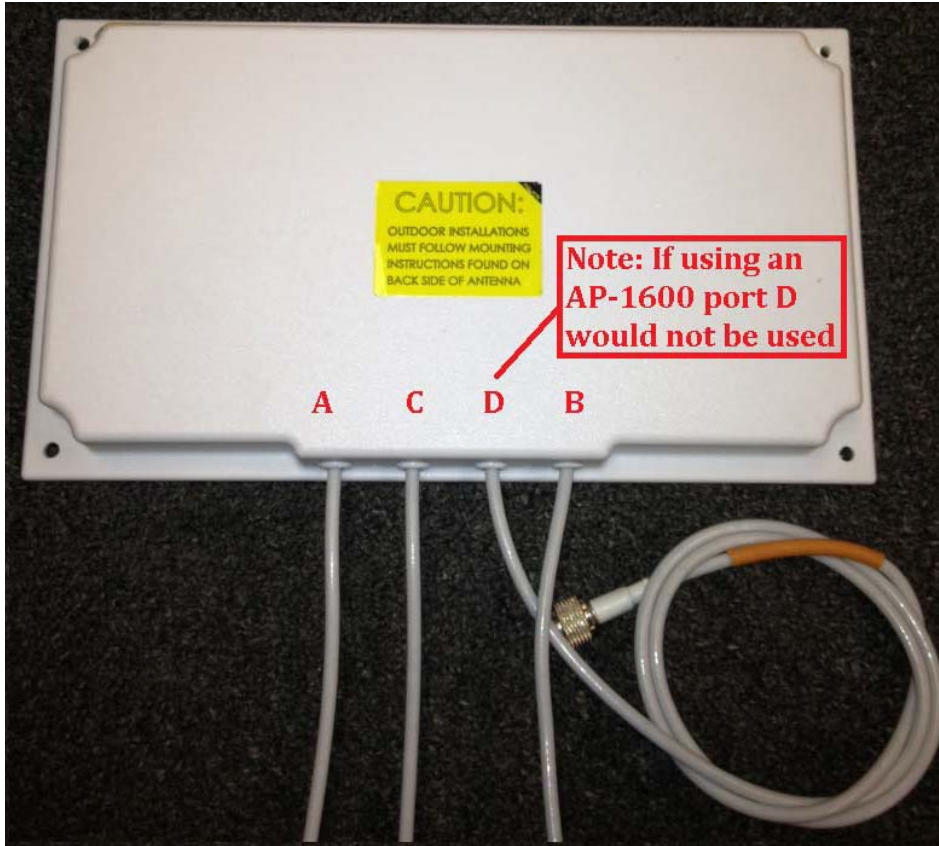
Figure 49 6 dBi Patch Antenna – While Not Critical, Ideally Ports “A” and “B” are Used on the ends.
