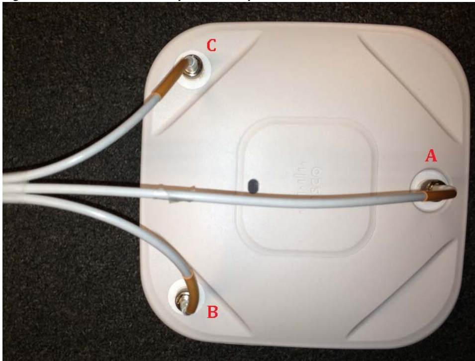
Figure 50 AP 1600 Note port “A” is Spaced Furthest from “B” and “C” for Best Diversity
