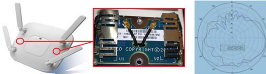
AP-3600e antenna system with module The Radio module has three internal antennas Note: AP-3600e when using directional antennas .11ac clients remain Omni-Directional
