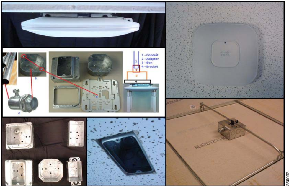
Figure 26 Mounting an AP onto an Electrical Conduit Box (Ceiling T-Bar or Conduit)
