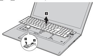
**6** Reconnect the keyboard connector and install the new keyboard. Push the keyboard in gently until it clicks into place.
