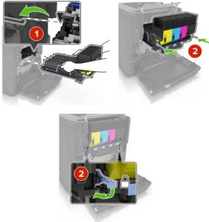
**11** Insert the waste toner bottle.
