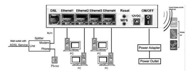
Notes: Without the splitter and certain situation, transient noise from telephone can interfere with the operation of the Router, and the Router may introduce noise to the telephone line. To prevent this from happening, a small external splitter must be connected to each telephone.
