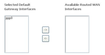
7. Get DNS server information from the selected WAN interface or enter static DNS server IP addresses. If only a single PVC with IPoA or static MER protocol is configured, you must enter static DNS server IP addresses.
