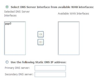
11. Make sure that the settings below match the settings provided by your ISP. Click on the Apply/Save button to save your configurations and reboot the ADSL router.
