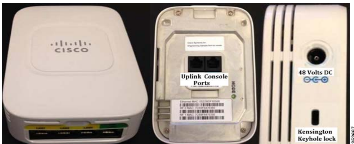
Figure 3 AP-702 Ethernet Switched Ports
