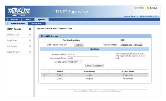
The TLNETCARD supports SNMP protocol and SNMP NMS (Network Management System), which are commonly used to monitor network devices. To prevent unauthorized access, the NMS IP addresses community strings and access levels for authorized users can be specified. The maximum number of IP entries is 256.
