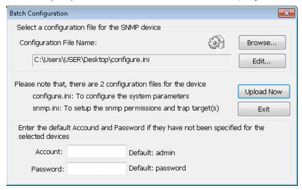
Step 7: Click on the Upload Now button. A notification appears when the process is complete.
