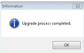
**Note:** The TLNET Configurator will not automatically show the updated firmware version in the Device List. Exit, then re-launch the TLNET Configurator to confirm the selected devices successfully uploaded the new firmware. The update can also be confirmed in the TLNET Supervisor interface of each device in the **Monitor** >> **About** tab.
