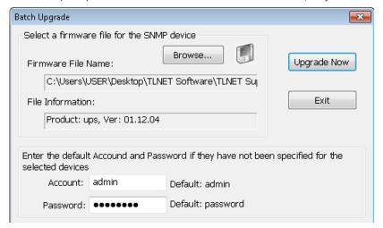
**Step 5:** Click the **Upgrade Now** button. A progress bar will indicate the upgrade status for each TLNETCARD sequentially. An information window will denote when the upgrade has been completed. Click **OK**.
