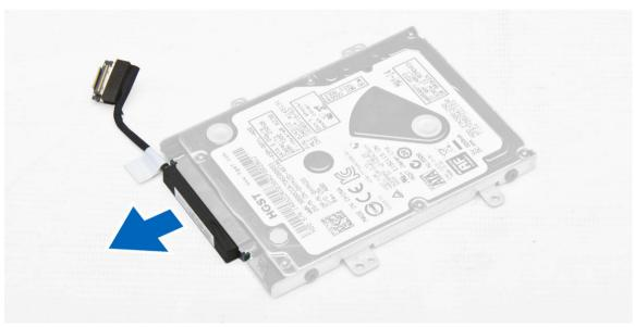
**4.** Remove the screws that secure the hard drive bracket to the hard drive [1] and lift the hard drive from the hard drive bracket [2].
