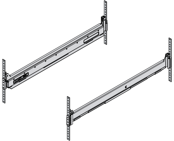
Figure 29: Round Hole Adapter and Rails Installed in a Rack
