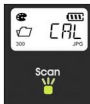
5. Press the [**Scan**] button. The calibration chart will be fed through.
