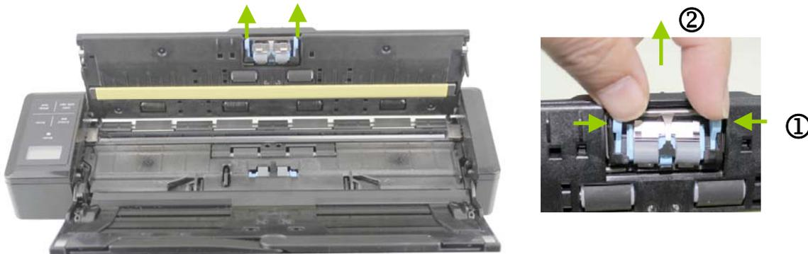
4. Hold two arms of the separation pad with two fingers and attach the new separation pad to the scanner.
