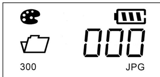
After the scanner is turned on, the LCD displays the default scan settings, Resolution: 300 dpi, Color mode: color, File format: JPG.
