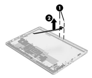
Reverse this procedure to replace the POGO connector.
