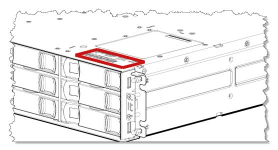
The following illustration provides a representative example of a serial number label on a chassis.
