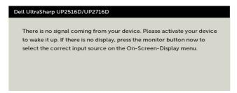
If either DP, mDP, HDMI/MHL 1 or HDMI/MHL 2 input is selected and the corresponding cable is not connected, a floating dialog box as shown below appears.
