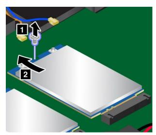
7. Align the contact edge of the new wireless WAN card with the key in the slot. Then carefully insert the new wireless WAN card into the slot. Then install the screw to secure the card.
