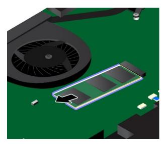
7. Align the contact edge of the new M.2 solid-state drive with the key in the slot. Then carefully insert the M.2 solid-state drive into the slot at an angle of about 20 degrees. Pivot the M.2 solid-state drive downward until it snaps into place. Ensure that the M.2 solid-state drive is firmly installed in the slot and cannot be moved easily.
