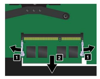
6. Place the notched end of the new memory module toward the contact edge side of the memory slot. Then insert the memory module 1 into the slot at an angle of about 20 degrees. Pivot the memory module downward until it snaps into place 2. Ensure that the memory module is firmly installed in the slot and cannot be moved easily.
