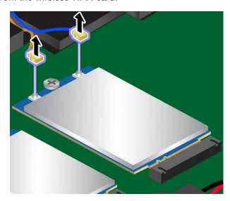
6. Remove the screw. The wireless WAN card is released from the secured position and pivots upward. Then remove the card.
