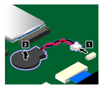
6. Install the new coin-cell battery 1 and attach the connector 2.
