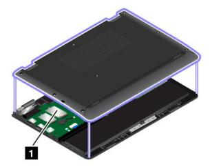
Note: For the user-replaceable wireless module, ensure that you use only Lenovo-authorized wireless modules for the computer. Otherwise, an error message will be displayed and the computer will beep when you turn on the computer.
