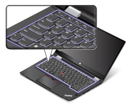
When you rotate the computer display from 190 degrees to 360 degrees, the frame of the keyboard travels upward for about 2.0 mm (0.08 inch). The following illustration shows that the keyboard frame travels upward.
