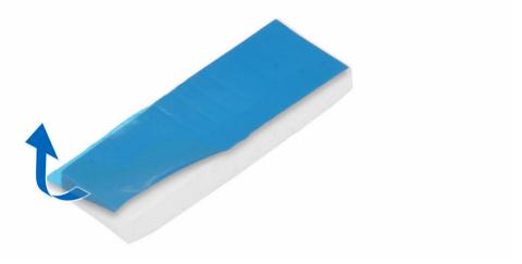
**4.** Place the rubber on the system board [1] and peel the adhesive tape (pink) from the rubber [2].
