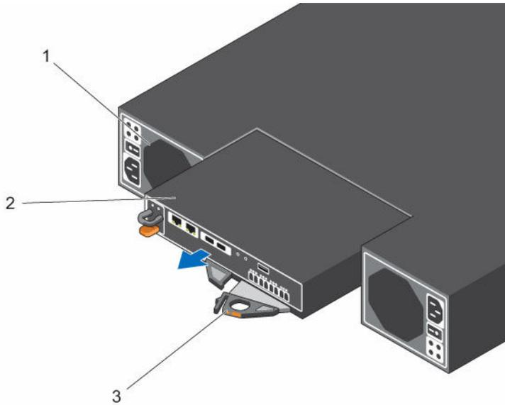
**Figure 25. Replacing a Storage Controller**
