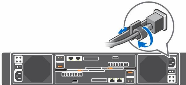
**Figure 15. Securing the Power Cable**
