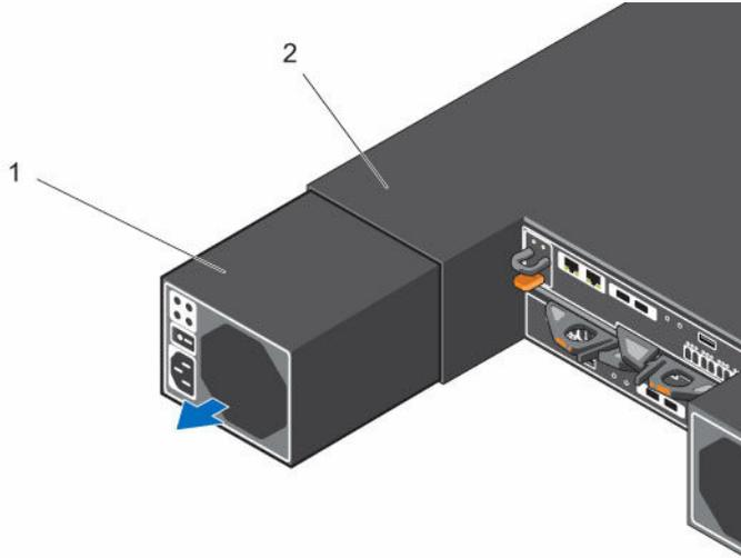
**Figure 14. Removing a Power Supply/Cooling Fan Module**
