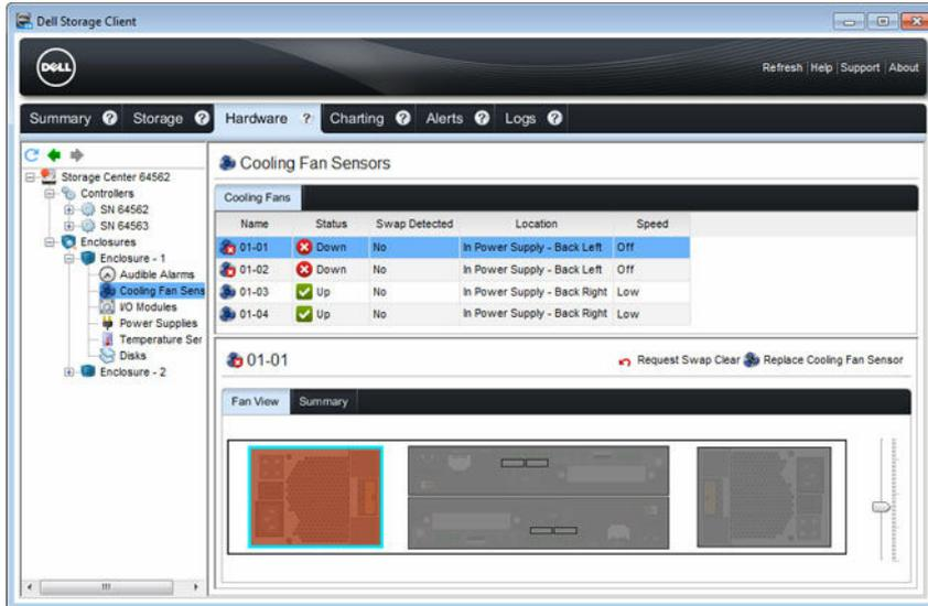
Figure 13. Rear View of the Enclosure Showing the Failed Cooling Fan
