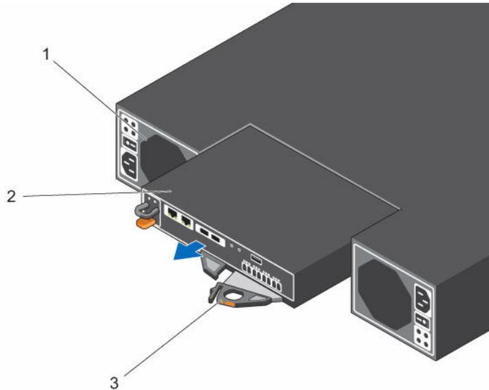
**Figure 26. Replacing a Storage Controller**
