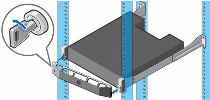
Figure 9. Replacing the Front Bezel
