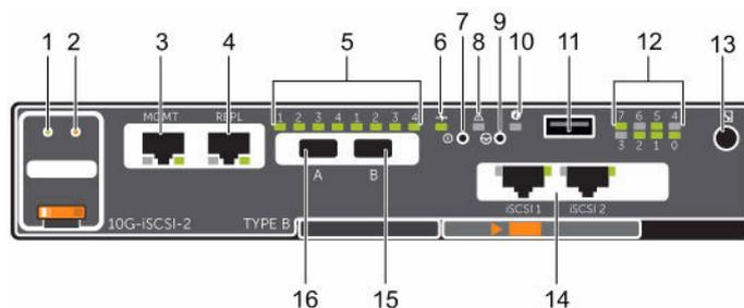
Figure 6. SCv2000/SCv2020 Storage System Storage Controller with Two 10 GbE iSCSI Front-End Ports
