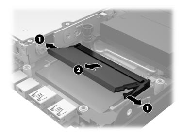
11. Slide the new SODIMM into the socket at approximately a 30° angle (1) then press the SODIMM down (2) so that the latches lock it in place.
