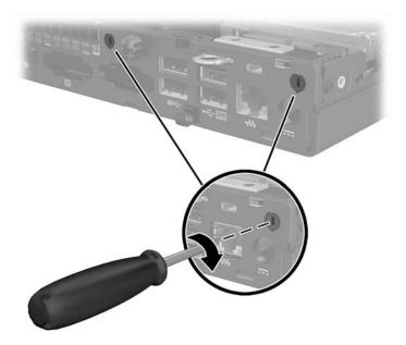
**18.** Feed the external antenna cable through each hole and screw the antenna into position.
