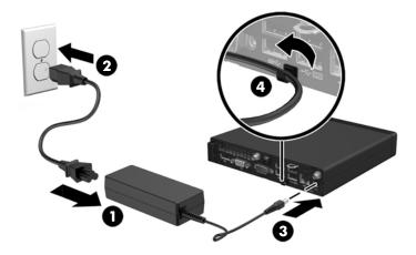
**CAUTION:** Failure to secure the AC adapter cord with the retainer clip may result in the adapter cord becoming disconnected and loss of data.
