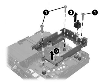
**14.** Locate the SSD on the system board.
