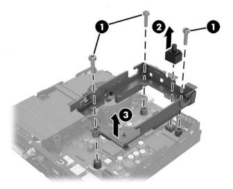
**14.** Locate the battery and battery holder on the system board.
