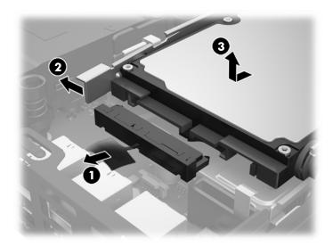
To install a HDD, you must transfer the silver and blue isolation mounting guide screws from the old HDD to the new HDD.
