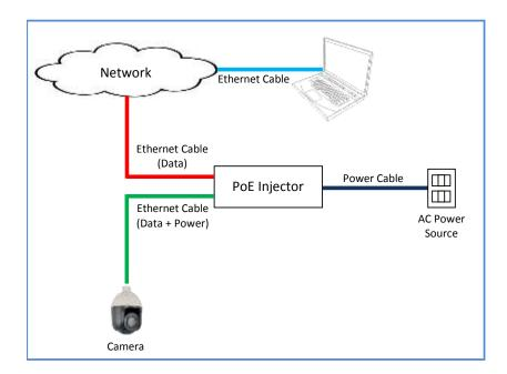
**NOTE:** Use only the supplied power adapter and power cord that came with the camera or the optional High PoE Injector available for purchase. Using other accessories not approved by the manufacturer may cause damage to the equipment.
