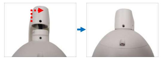
2. Attach the screws included in the camera package to secure the camera.
