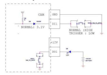
Consequently, to connect a second DI or DO device, use the GND and DI2 pins to connect the second DI device, and the 12V and DO2 pins for the second DO device.
