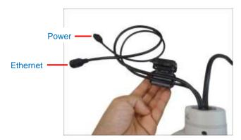
3. Snap the ferrite core to secure it on the cable.
