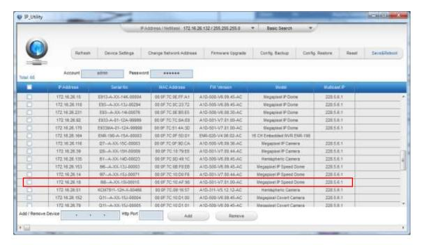
The camera model name is shown on the list. Click on the IP address to automatically launch the default browser of the PC with the IP address of the target camera already filled in the address bar of the browser.
