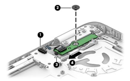
Remove the power button board from a 15" computer:
