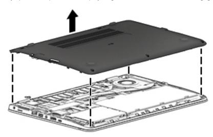
Reverse the removal procedures to install the bottom cover.
