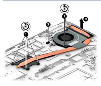
NOTE: The thermal material must be thoroughly cleaned from the surfaces of the heat sink and the system board components each time the heat sink is removed. Replacement thermal material is included with the heat sink, processor, and system board spare part kits.
