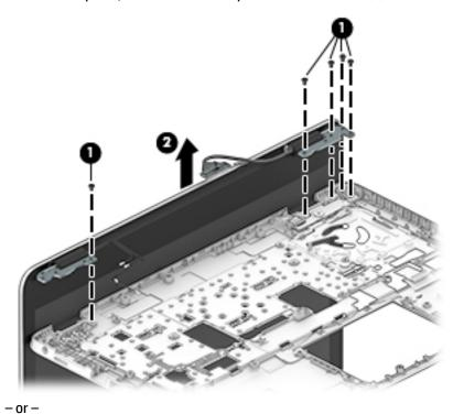
On a 15" computer, remove the 4 Phillips PM2.5×5.0 screws (1) from the display hinges.
