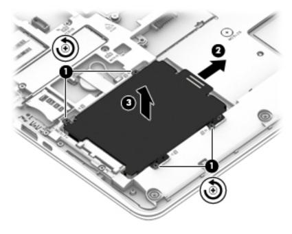
To remove the hard drive cover and bracket from the hard drive, lift the Mylar cover up off the drive, remove the 4 Phillips PM3.0×3.0 screws (1) that secure the bracket to the drive, and then lift the bracket up and off the hard drive (2).
