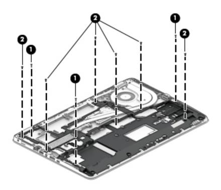
On 14" computers, remove 9 Phillips PM2.5x5.0 screws (1), and then remove the base plate from the computer (2).
