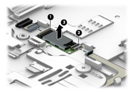
Reverse the removal procedures to install the NFC module.
