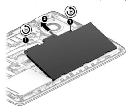
Reverse the removal procedures to install the battery.
