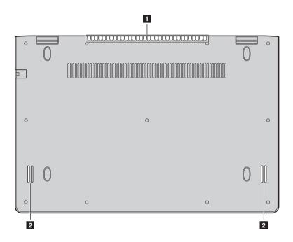
Ventilation slots Dissipate internal heat.
