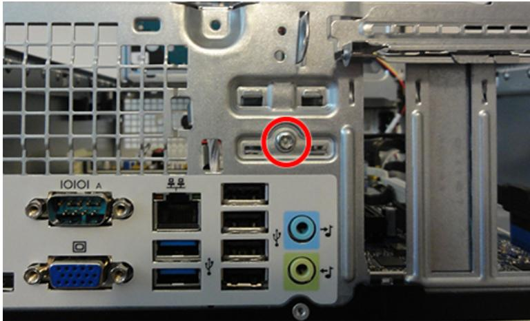
4. From the inside of the computer, lift the hood lock out of the computer..
