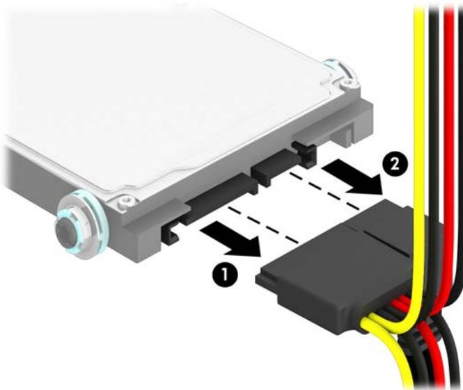
5. Pull outward on the release lever at the rear of the drive (1) then slide the drive back until it stops and pull it down and out of the drive bay (2).
