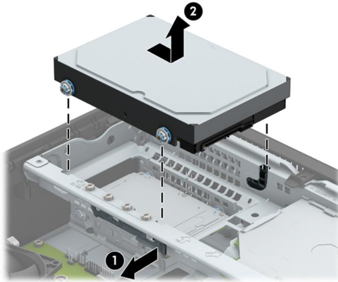
5. To install a hard drive, you must transfer the mounting screws from the old hard drive to the new hard drive.
