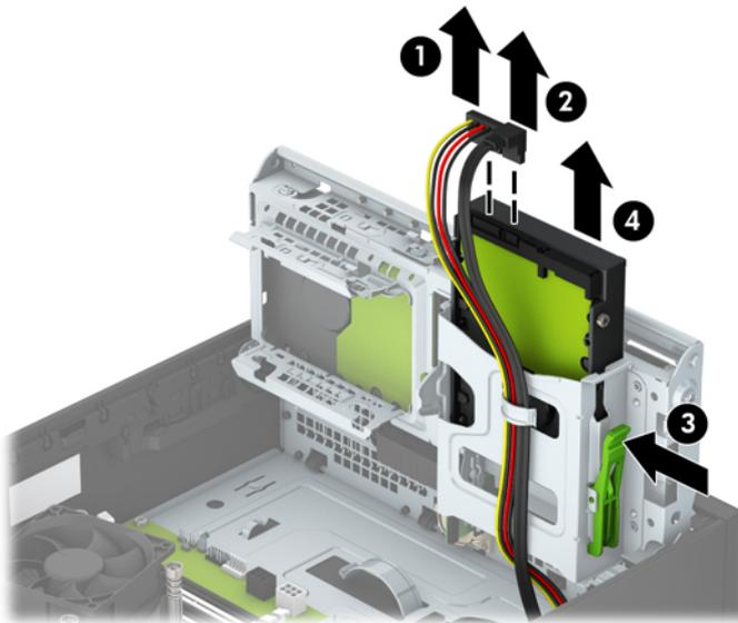
5. If you are installing a new drive, refer to [Installing a secondary 3.5-inch hard drive on page 40](#). If you are not installing a new drive, rotate the drive cage down and replace the access panel.
