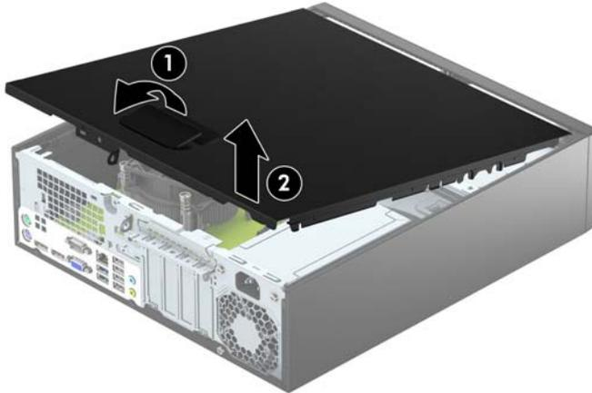
To install the access panel, reverse the removal procedure.
