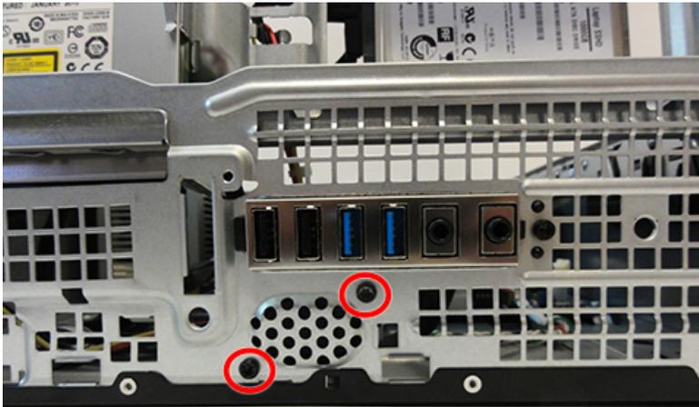
6. From the inside of the chassis, disconnect the speaker cable from the white system board labeled SPKR, and remove the speaker from the chassis.
