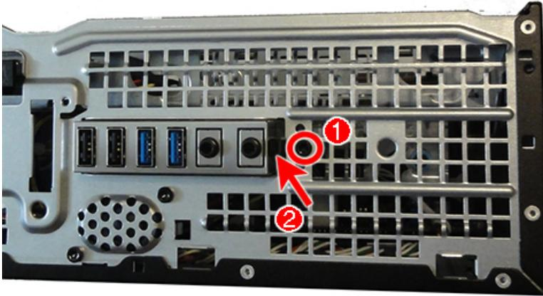
9. Remove the front I/O assembly from the inside of the computer.
