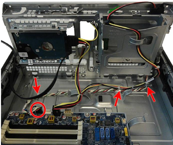
7. Remove the power switch assembly from the inside of the computer.
