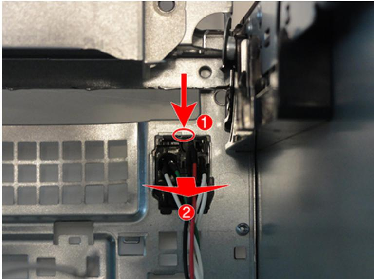
6. Remove the cable from the clips built into the bottom of the chassis, then and disconnect the power switch cable from the system board connector labeled PB/LED.
