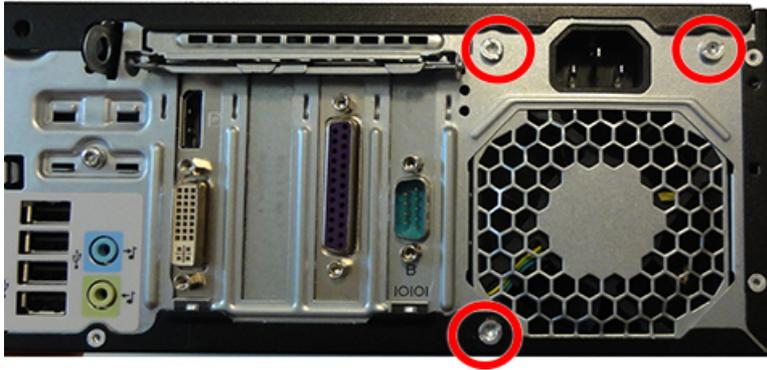
6. From the inside of the chassis, push the release lever at the front of the power supply (1), slide the power supply forward, and then remove it from the chassis (2).
